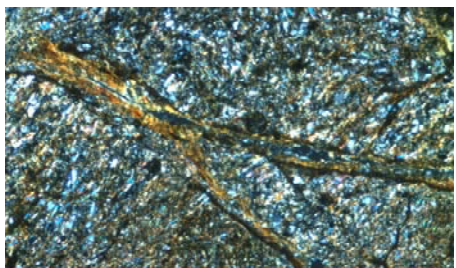
Figure 4. Clay illuviation in slates: clay infillings in cracks and clay coatings in pores (1.68 mm width, XPL).
