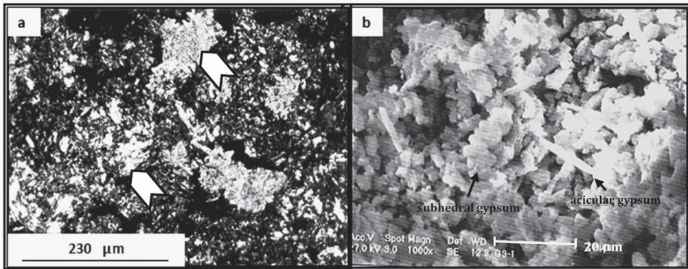
**Figure 3.** a) Fine grained xenotopic gypsum in transmitted light (XPL), b) subhedral and acicular gypsum crystals (SEM). 2Byz horizon of Pedon 4.
