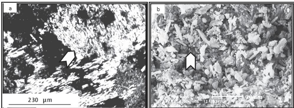
**Figure 4.** Fibrous bassanite, alteromorph after xenotopic gypsum a) in transmitted light (XPL), b) SEM of fine bassanite resulting from gypsum dehydration. 2Byz horizon of Pedon 2.
