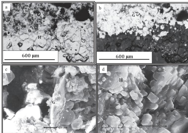
**Figure 6.** Gypsum (G) and halite (H) crystals in petrogypsic/salic horizon as coatings and infillings a) PPL, b) XPL, c) lenticular gypsum (SEM). d) halite (SEM). 3Byzm horizon of Pedon 2.
