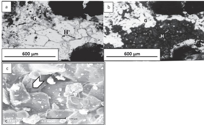
**Figure 5.** Anhydral gypsum (G) coating and halite (H) infilling. a) PPL and b) XPL, c) cubic halite crystals (SEM). 3Byzm horizon of Pedon 1.
