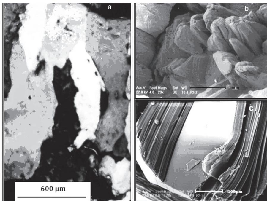
**Figure 8.** Palisade fabric in gypsum pendants. a) transmitted light (XPL) (the higher interference colours are caused by uneven thickness of the thin section); b and c) SEM images. Note the clear cleavage planes of the gypsum. 4Byz horizon of Pedon 2.
